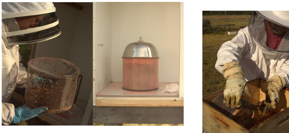
Figure 2. Dusting of bees using vacuum chamber in the field. Bees were shaken from frames into a screen cage. The cage was placed inside one of the chamber domes. A vacuum was drawn and released, filling the dome and cage with suspended dust. The cage with dusted bees was then returned to the source colony.
